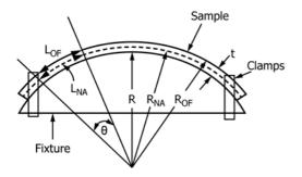
R = radius of jig  $\theta$  = arbitrary angle  $R_{NA}$  = radius of neutral axis R<sub>OF</sub> = radius of outer fiber t = thickness of specimen
